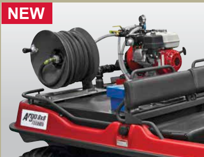
NEW NEW Fire fighting platform: 75 gallon tank, 5 gallon foam cell, 6 hp Honda engine, fire pump, booster hose and forestry nozzle.
