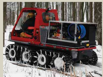
The all season ARGO can be outfitted with customized equipment for firefighting.
