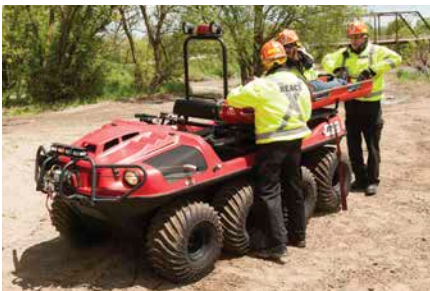
An ARGO equipped with search and rescue apparatus can reach and evacuate injured in remote terrain.
