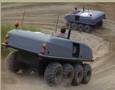
Fully autonomous ground vehicles (unmanned or with operator) used for perimeter patrol, surveillance, fire fighting, and re-supply.
