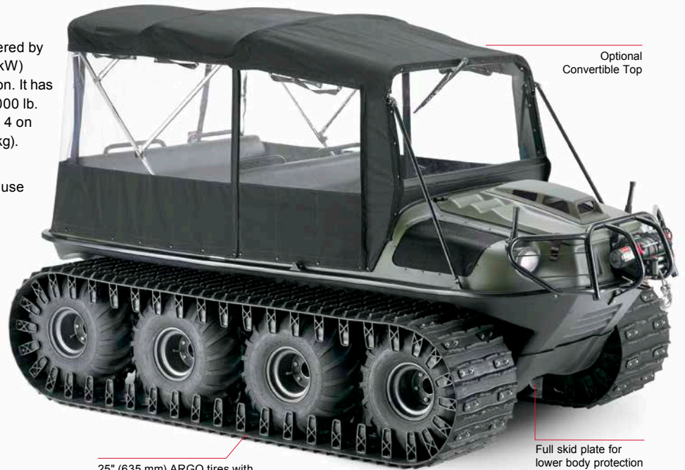
25" (635 mm) ARGO tires with proprietary tread design shown with optional rubber tracks
