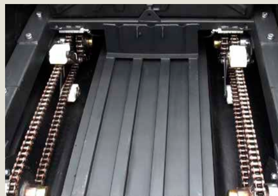
3" Tubular frame and reversible chain adjusters
