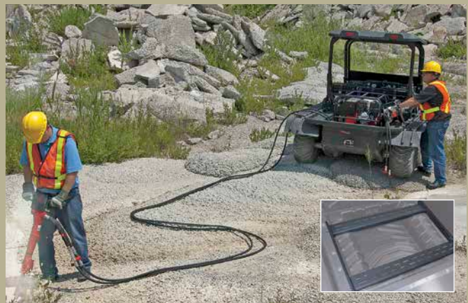
Hydraulic power pack made by Chicago Pneumatic. Installation with quick connect ARGO Universal Mounting System (Inset).
