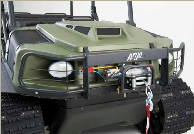
Halogen headlights, optional brushguard, 4,500 lb. (2,041 kg) power winch (optional) and skid plate for lower body protection.
