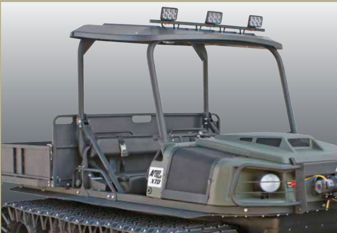
Optional, certified ROPS for two or four passengers is available with hard top for sun / rain protection and a light bar to add auxiliary lighting.
