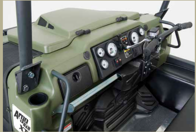
Multi-position steering system, instrumentation panel and convenience package (two cup holders, two storage compartments and two 12 volt outlets).
