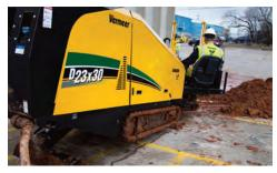
COMPACT YET POWERFUL. The D23x30 S3 features a short, narrow design, while its 100 hp (75 kW) Deutz engine offers the power operators need when working in tough ground conditions.
