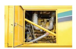
**ENGINE POWER.** A C27 Tier 4F engine provides 950 hp (708 kW) of power to meet your jobsite demands.
