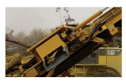
**OVERBAND MAGNET.** An optional, overband helps remove ferrous material from the end product.
