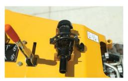
PORTA BORING. Easily transition from plowing to boring under driveways, sidewalks and other obstacles with an optional Porta Bore attachment.
