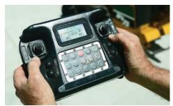
**REMOTE CONTROL.** A remote control gives you 360-degree control of the machine, providing greater maneuverability on tight jobsites, as well as visibility to the complete worksite and to avoid potential obstacles or obstructions that may be difficult to operate with conventional controls.
