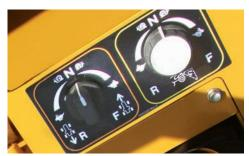
**GROUND DRIVE POWER.** An electronically controlled hydraulic pump provides operators with more precise control and greater efficiency in comparison to machines with manually controlled pumps.
