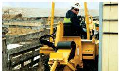
MANEUVERABILITY. A class-leading compact turning diameter allows the RTX450 to perform in narrow jobsites - especially in residential areas.
