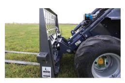
FULL-SIZED ATTACHMENT PLATE. The full-sized attachment plate on the ATX960 is compatible will full-sized articulated loader attachments. The ATX960 can be fitted with various authorized attachments to meet the jobsite need, may that be for snow removal, landscaping, logging and tree care work, or various other Vermeer applications.
