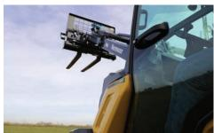
TELESCOPIC BOOM. The telescopic boom on the ATX960 extends 49.5 in (125.7 cm) for loading materials to a dump height of 126 in (320.04 cm) in hinge pin height. The telescopic boom can also aid in dumping material over the backside of a retaining wall or grabbing material over an obstruction.
