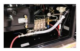
WATER SYSTEM. The water system is rated for 19.4 gpm @ 3,000 psi (73.4 L/min @ 20,684 kPa).
