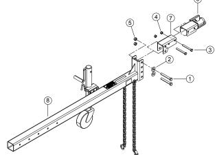
Figure 2.1, Non-CE Compliant Hitch Assembly
