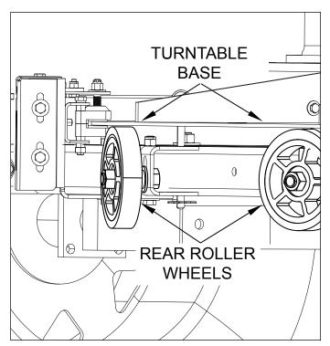
Figure 2.10, Rear roller wheel adjustment
