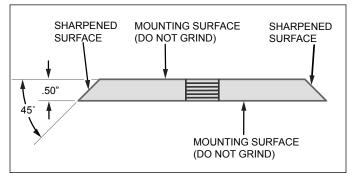
Figure 5.2, Chipper Blade Surfaces
