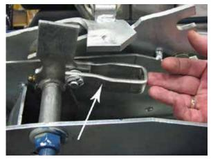
Figure 2.2, Remove this clevis on 50mm coupler
