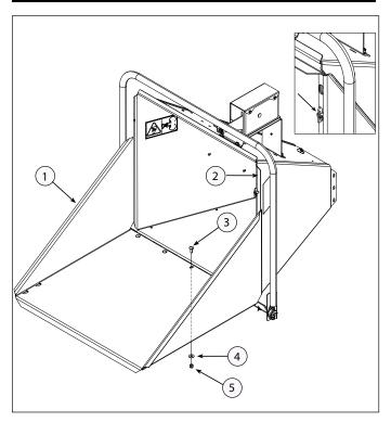
Figure 2.6, Attaching the extension tray
