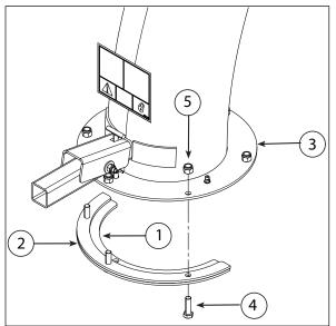
Figure 2.7, Attach clamp ring and spacer
