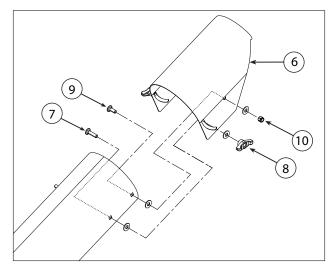
Figure 2.9, Attach discharge deflector
