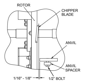
Figure 5.3, Chipper Blade/Anvil Clearance
