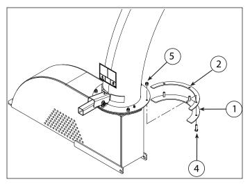
Figure 2.8, Attach discharge tube
