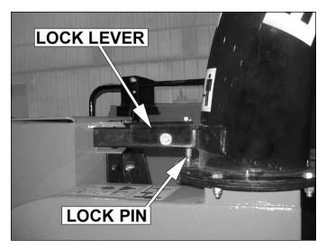
Figure 4.1 - Directing the Discharge Tube/Cap.
