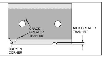
• The base of the cutting edge is worn or has been resharpened so that it no longer extends past the chipping slot (see below).
