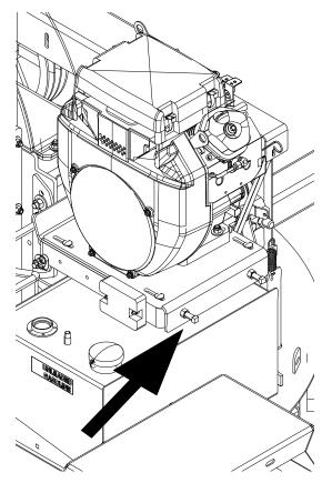
Figure 5.5, The tension bolts are pointed out in the drawing.
