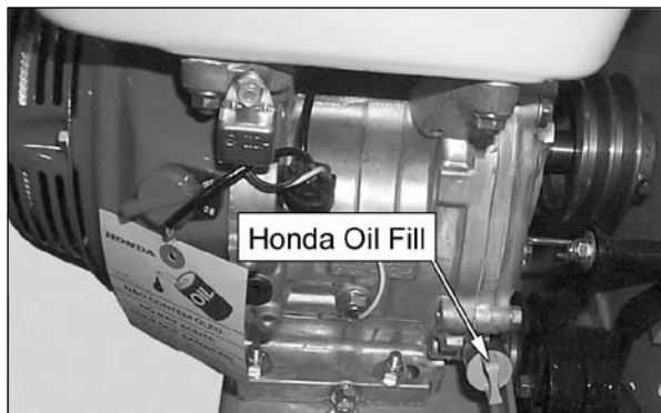
Figure 2.2 - Honda Oil Fill
