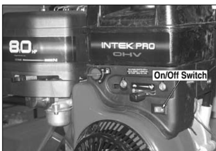
Figure 3.8 Briggs Commercial On/Off Switch
