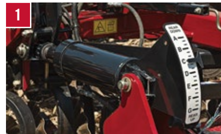
Hydraulic fore/aft control: maintain consistent agronomic output
