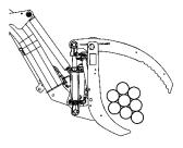
E. Close the upper jaw to secure load. Lift slightly the load.
