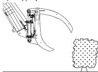
B. Rotate front of the accessory down. Lower the accessory until upper and lower jaw become in contact with the ground on each side of the bushes.
