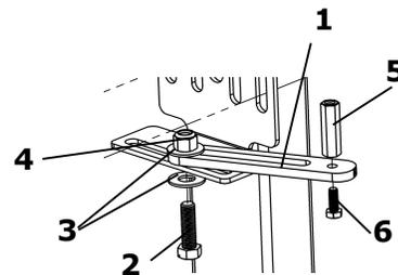
**NOTE:** Make sure the coupling nuts are perpendicular to the ground. If this is not the case, it is possible to bend the rear support, but it is recommended to wait until the cab has been installed in the right position to do this adjustment.
