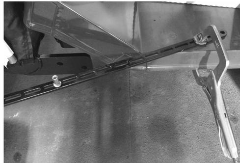
**NOTE:** Make sure the coupling nuts are perpendicular to the ground. If this is not the case, it is possible to bend the support, but it is recommended to wait until the cab has been installed in the right position to do this adjustment.
