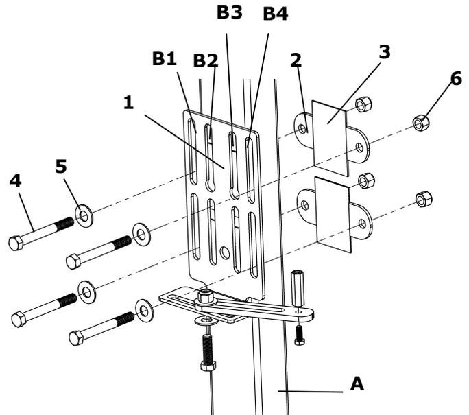
Install the rear support (item 1) on the rear support bracket installed in the preceding step) with a bolt M10 X 30 (item 2), 2 flat washers 7/16" (item 3) and nuts (item 4) as shown.
