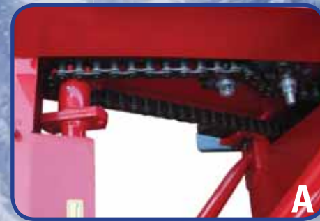
A. SAFETY BOLTS ON DRIVING SHAFT, 2 SPROCKETS ONE WITH SPRING AND ONE ADJUSTABLE
