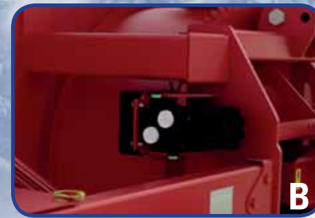
B. HYDRAULIC DRUM ROTATION WITH GEAR AND MOTOR WITH CUSHION VALVE (ON TR MODELS)
