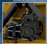
Forced lubrication system with oil level
