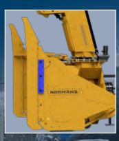
Directional hydraulic lateral blades in Hardox 450 steel and truck diverter
