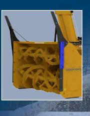
Fixed lateral blade in Hardox 450 steel and truck diverter
