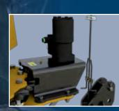
Hydraulic motor for chute with reducer and protected by a cushion valve
