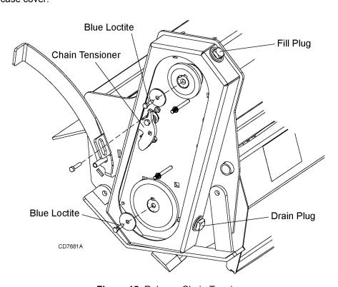
Figure 15. Release Chain Tension
