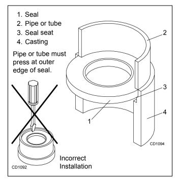
Figure 14. Seal Installation
