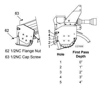
Figure 6. Tiller Depth Adjustment
