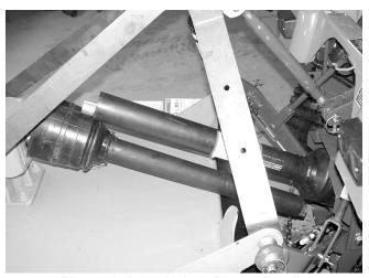
Figure 1. Drive Halves Placed Parallel
