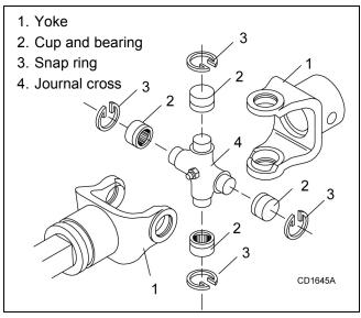
Figure 16. Universal Joint Parts Breakdown
