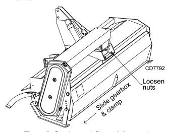
Figure 8. Gearbox and Clamp Adjustment
