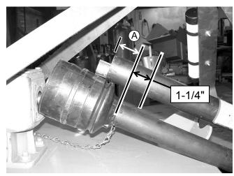
Figure 2. Determine Shield Length
