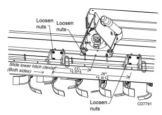
Figure 7. Clevis Hitch Adjustment
