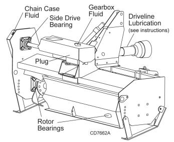
Figure 10. Lubrication Points
