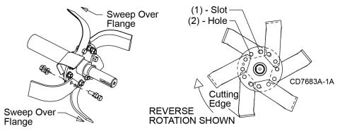
Figure 13. Six Blade Installation
