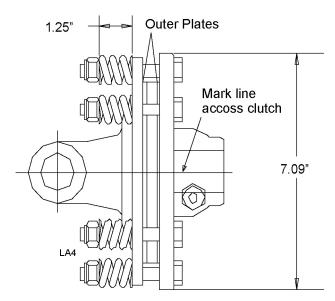
Figure 11. Slip Clutch Adjustment
