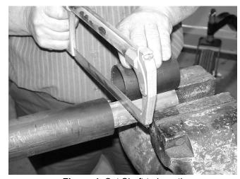
Figure 4. Cut Shaft to Length
