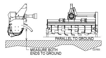
Figure 5. Leveling the Tiller
