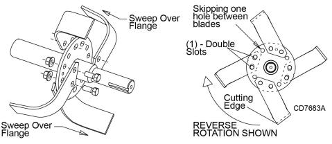
Figure 12. Four Blade Installation
