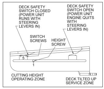
Figure 12. Power Tilt Deck Safety Switch Layout
