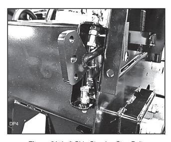
Figure 21. Left Side Steering Stop Bolts
