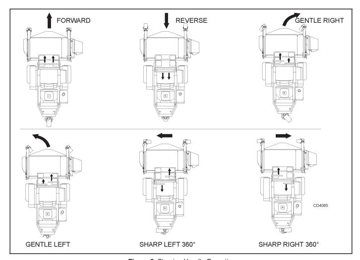
Figure 2. Steering Handle Operation
