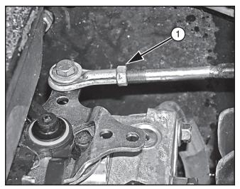
Figure 10. Jam Nut on Linkage Rod, Left Pump
