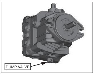
Figure 4. Left Pump Dump Valve
