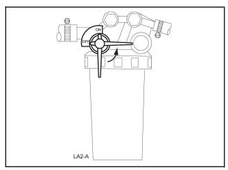
Figure 3. Manual Shut-Off Valve
