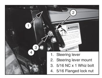
Figure 20. Steering Handle Adjustment
