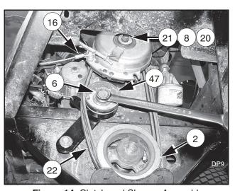
Figure 14. Clutch and Sheave Assembly
