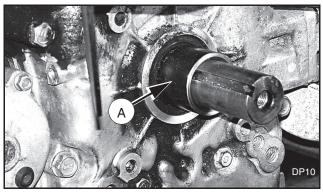
Figure 16. Clutch Spacer Installed
