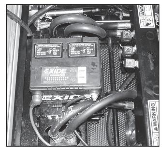
Figure 9. Battery Located under Seat
