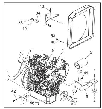
Figure 13. Rubber Isolator & Radiator Mount
