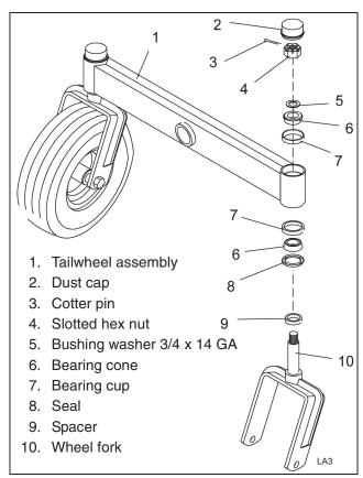
Figure 7. Tailwheel Assembly (Typical)
