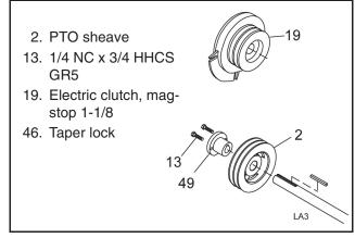
Figure 17. Align Clutch & PTO Sheave
