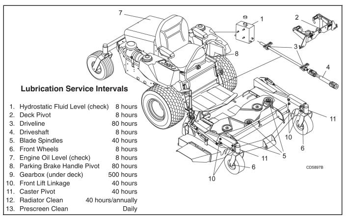
Figure 6. Lubrication Diagram
