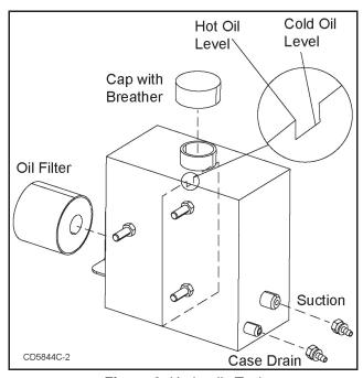
Figure 8. Hydraulic Tank
