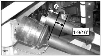
Figure 5. Determine Shield Length
