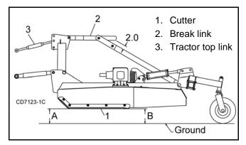
Figure 8. Cutting Height Adjustment
