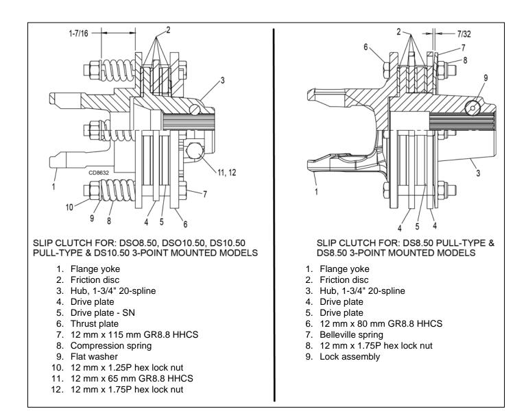
Figure 13. Slip Clutch Assembly
