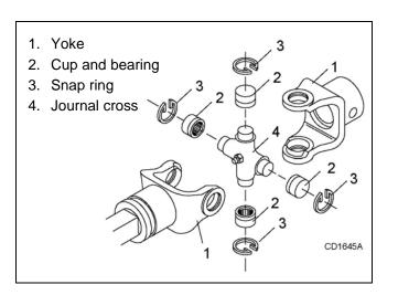
Figure 22. Universal Joint Exploded View
