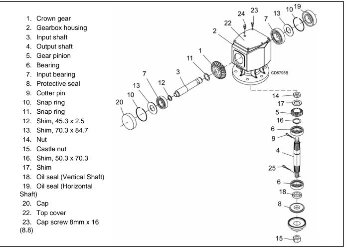
Figure 14. Spindle Gearbox Assembly
