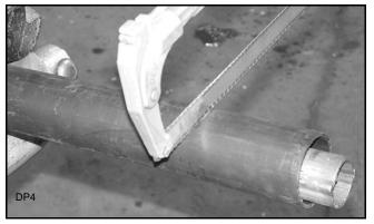
Figure 6. Cut Shield
