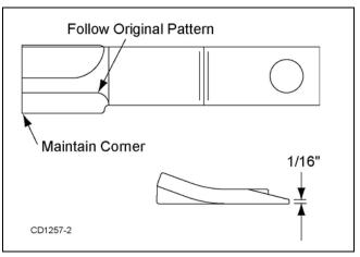
Figure 12. Sharpen Blade Cutting Edge
