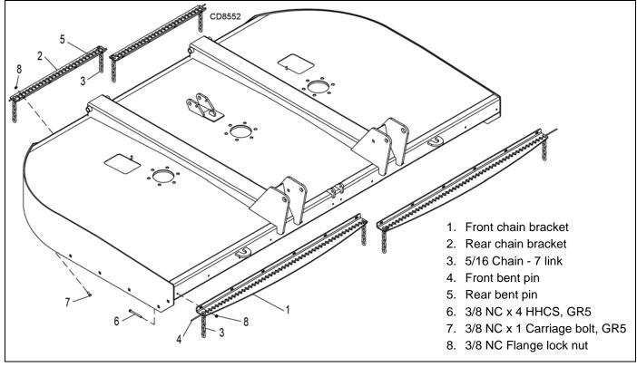
Figure 32. Optional Chain Shielding Installation
