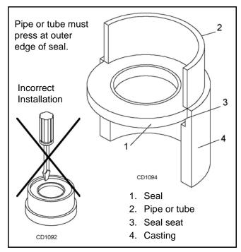
Figure 13. Seal Installation
