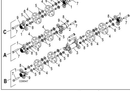
The drives between the center and side gearboxes contain rubber shock-absorbing discs. To service or remove the side drives or remove a gearbox, the flexible coupling must be disassembled. See page 25 for rubber disk replacement.
