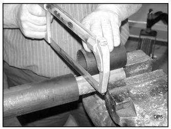
Figure 7. Cut Shaft to Length
