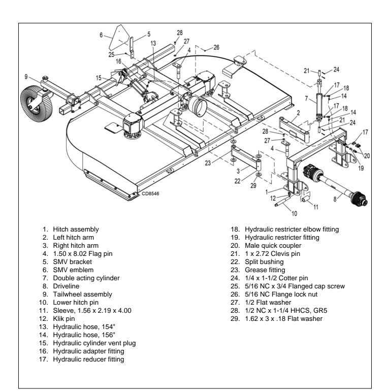
Figure 30. DSO8.50 & DSO10.50 3-Point Mounted Cutter Assembly
