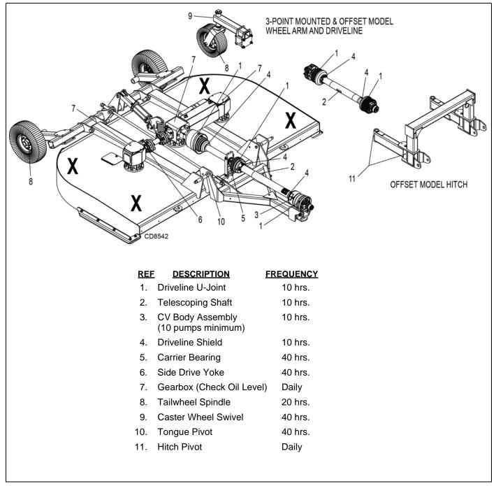
Figure 10. Jackstand Placement and Lubrication Points
