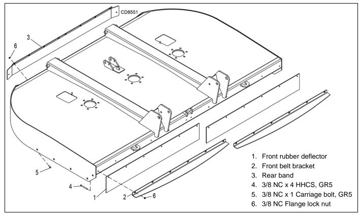
Figure 31. Rubber Belt Shielding Installation
