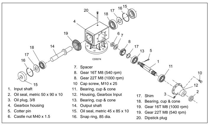
Figure 15. Splitter Gearbox Assembly
