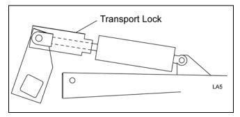
Figure 9. Transport Lock Operation
