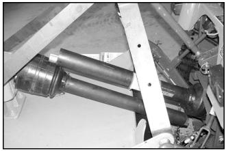
Figure 4. Drive Halves Placed Parallel
