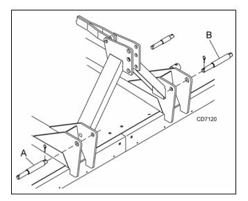
Figure 2. 3-Point Mounting Positions
