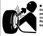
■ Explosive separation of tire and rim parts can cause serious injury or death. Release all air pressure before loosening bolts.
