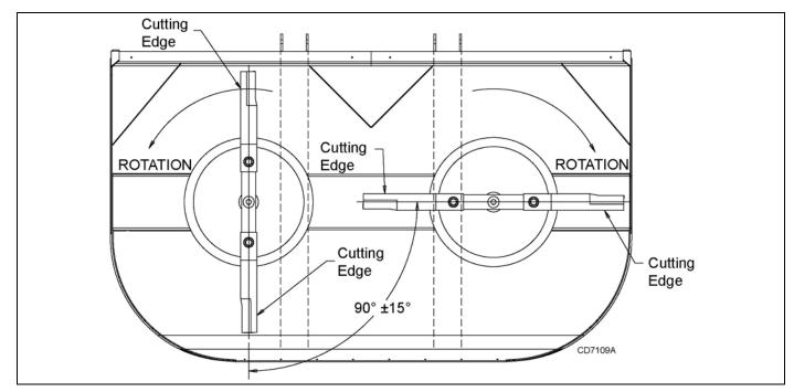
Figure 21. Crossbar Timing - Bottom View
