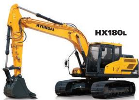
**Net Power** Perkins 1204F SAE J1349 / 128 HP (96 kW) at 2,050 rpm
