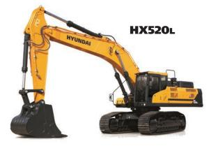
**Net Power** Scania DC13 SAE J1349 / 424 HP (316 kW) at 1,900 rpm
