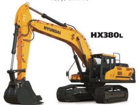
**Net Power** Cummins QSL9 SAE J1349 / 300 HP (224 kW) at 1,650 rpm
