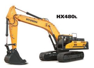
**Net Power** Scania DC13 SAE J1349 / 424 HP (316 kW) at 1,900 rpm
