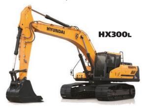
**Net Power** Cummins QSB6.7 SAE J1349 / 230 HP (171 kW) at 1,950 rpm
