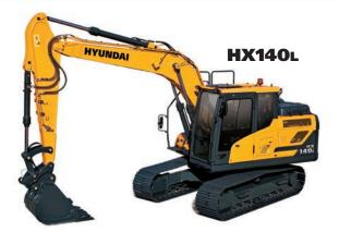
**Net Power** Perkins 1204F SAE J1349 / 116 HP (92.6 kW) at 1,950 rpm
