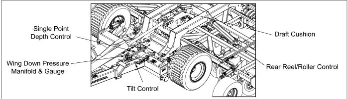
Figure 4-7: Operating Depths and Adjustments
