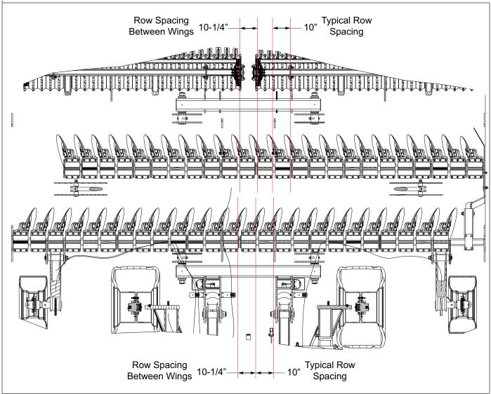
Figure 4-5: Lateral Adjustment of Gang Assemblies (2 of 2)
