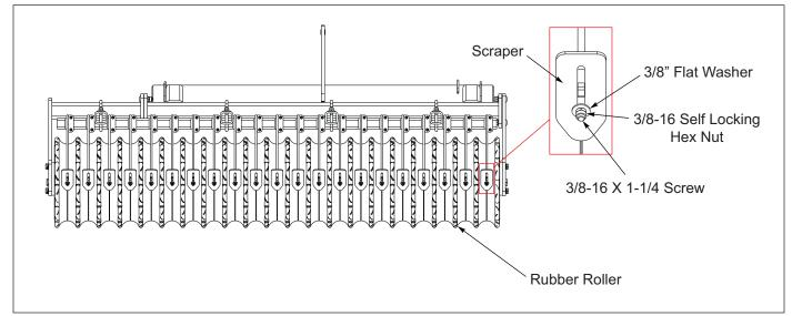
Figure 4-10: Rubber Roller Scraper Adjustment
