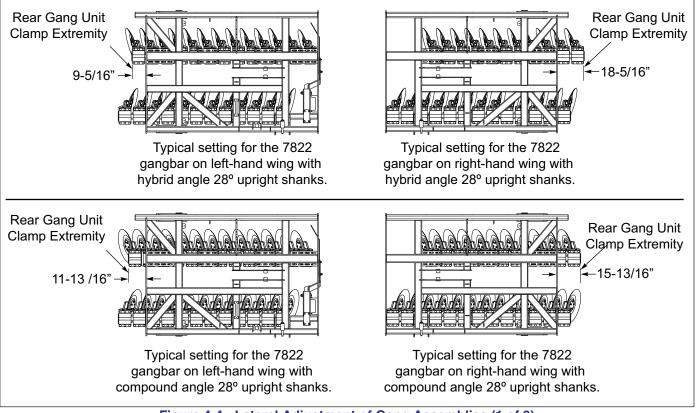
Figure 4-4: Lateral Adjustment of Gang Assemblies (1 of 2)
