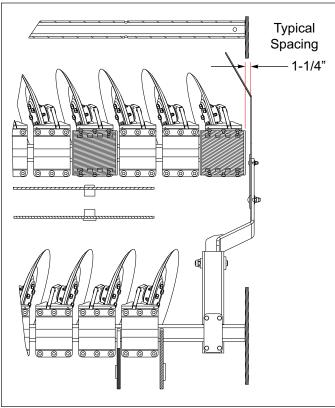
Figure 4-6: Adjusting the Blade Leveler
