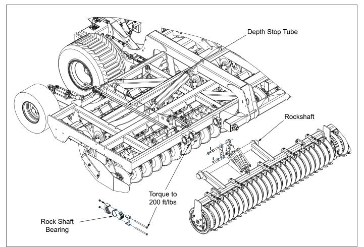
Figure 3-3: Rear Gauge Assembly
