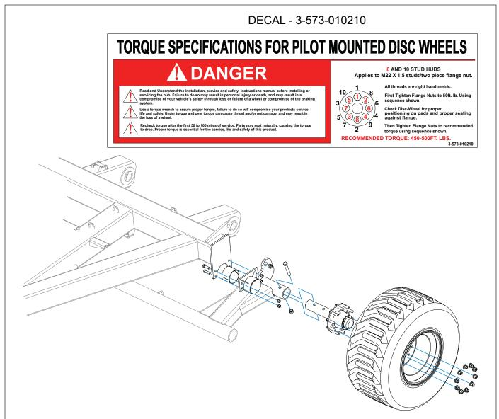
Figure 3-2: Tire and Wheel Installation
