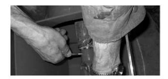
8. Slide clamp halves down to hopper and install the 3/8" x 1" (10 x 25 mm) bolts with flat washers and lock nuts. Adjust hopper to set flat (square) with the ground and tighten clamp bolts.
