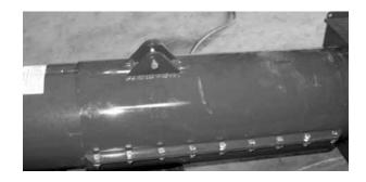
9. Install rubber hopper extension using the 1/4" x 1/2" (6 x 13 mm) carriage bolts provided.
