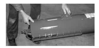
5. Slide hopper assembly onto auger.
