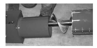
6. As the hopper is being slid over the auger, be sure to align hole in U-joint with hole in auger shaft (if present). On augers without a hole in the shaft, slide U-joint on shaft and use hole in U-joint as a pilot hole to drill shaft.
