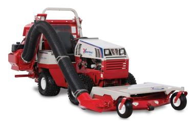
The Ventrac RV602 Vacuum Collection System is for grass and leaf collection, and it consists of three primary components:
