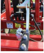
Control Makes it easy to adjust operating depth for varying field conditions or change from spring
