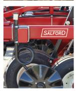
**Welded End Caps** 4 inch x 6 inch tubular steel frame and beam ends that are welded shut for increased durability and longevity.
