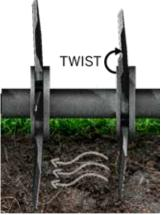
The HALO AerWay's wavy coulter blades run on either side of the tines, further sizing and mixing residue. The coulter and tine angles are also adjustable, allowing for straight residue cutting or more aggressive leveling power.
