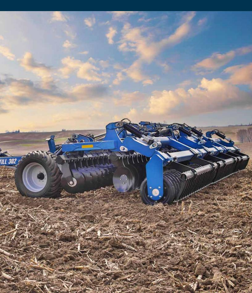
One tool for spring and fall tillage that quickly covers more acres, without creating compaction. Mach Till is a versatile, heavy built, low maintenance machine that prepares seed beds in the spring or incorporates residue in the fall. It operates at high speeds without creating compaction layers and produces an eye appealing finish. Agronomic benefits include nutrient cycling and improved soil density for water infiltration and reduced erosion.
