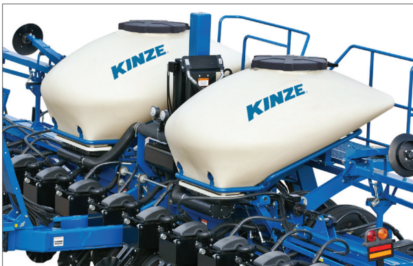
3665: Total bulk fill hopper seed capacity is 110 bushels.
