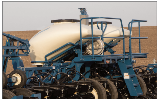
3605: Total bulk fill hopper seed capacity is 80 bushels.
