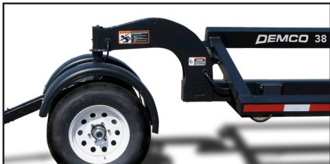
*The Tricycle front design allows for short turns and superior high speed towing capability*
