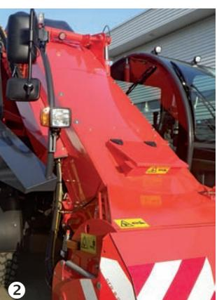
**③** To speed up loading, the width of the loading conveyor has been increased from 25" to 31". Feed is quickly transferred from the milling head to the tub and augers.
