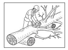
Don't cut with the saw overhead or aligned vertically with your body. If the saw should kick back, you may not have enough control to prevent possible injury.
