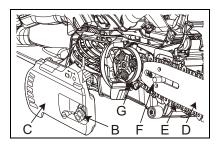
5. Mount guide bar (D) on stud (F) and slide toward clutch drum sprocket (G) to make saw chain (E) installation easier. Install saw chain around clutch drum sprocket and guide bar as shown, with saw chain cutters on top of guide bar facing forward.
