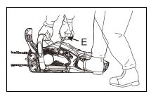
8. Turn choke control knob (D) clockwise to (OPEN | | choke position).
