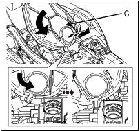
Insert the air filter cover (B) into the rear handle side and push it forward, then fix it with the filter cover latch (A).
