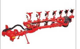
For added reliability, the structure is made using a large, machine-welded frame measuring approximately 7" x 7" (18 cm x 18 cm).
