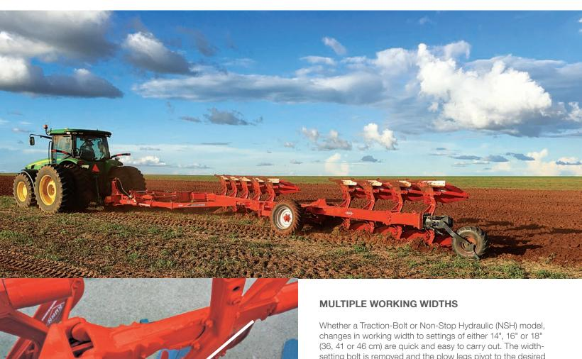
setting bolt is removed and the plow legs pivot to the desired width. The rear beam angle is changed in the same manner as the articulation joint-it moves positions corresponding to the required setting width.
