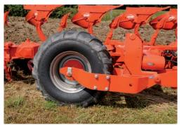
A stub axle mounted on tapered roller bearings With two telescopic, single-acting cylinders, makes this turning system incredibly reliable.
