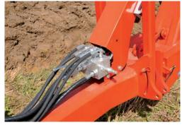
For more stability in transport, as well as frame protection during road travel, the lifting cylinder is equipped with hydropneumatic suspension.
