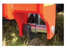
A wide range of hitch categories are available (Cat. 3, 4N, 4, Quick hitch 3 and 4N) to adapt to medium and high power tractors (135 to
