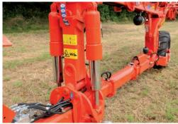
headland turns are jolt free. This also reduces stress on the tractor's lift arms allowing for optimum comfort during turns.
