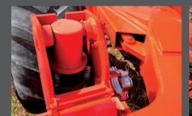
Spacers on the left cylinder provide plenty of Leveling is independent, left or right via stop depth. The number of spacers allows for a point of reference.
