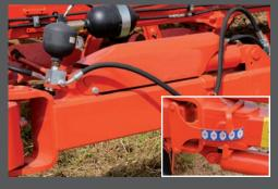
Adjusting the plow's offsets is done by a hydraulic cylinder (optional). This adjustment can go from 39" to 69" (99 to 175 cm). A gauge visible from the tractor allows for precision setting of the machine.
