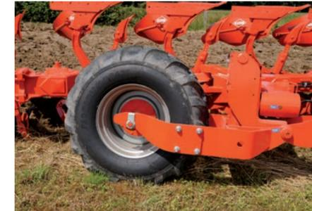
A stub axle mounted on tapered roller bearings makes this turning system incredibly reliable.
