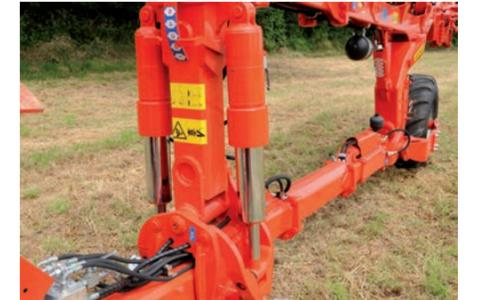
With two telescopic, single-acting cylinders, headland turns are jolt free. This also reduces stress on the tractor's lift arms allowing for optimum comfort during turns.
