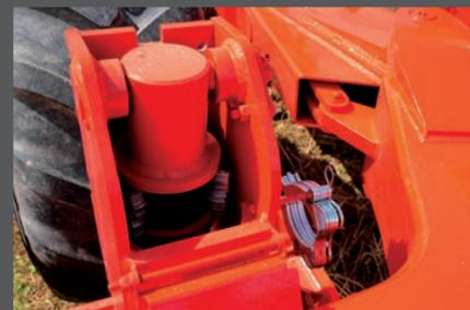
Spacers on the left cylinder provide plenty of depth. The number of spacers allows for a point of reference.
