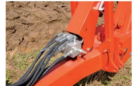
For more stability in transport, as well as frame protection during road travel, the lifting cylinder is equipped with hydropneumatic suspension.
