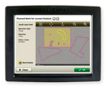
The pre-planned work task appears automatically on the cab display when the machine enters a field. All the operator has to do is confirm the details.
