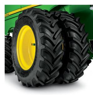
A 580/85R42 RIW dual tire option is available on a universal rim that can be dished in or out without axle spacers.
