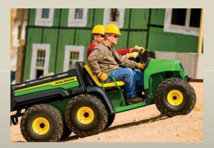
**Six-wheel design** Offers excellent traction, while remaining turf friendly. Includes standard traction assist.
