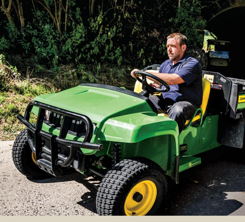
The 48-volt electrical system performs steady and smooth all day long.\* This transporter with zero operating emissions sports a 16.4 cubic foot (.46 cu m) capacityreinforced cargo box, the ideal solution for working inside large warehouses and buildings. The pick-up style tailgate and tie-down points make managing loads easier. For large loads, convert to flatbed mode by removing tailgate and side panels.
