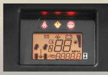
Easy-to-read dash panel lets you quickly scan your speed, gear position, and now, fuel level.
