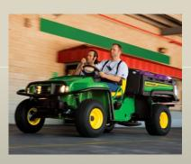
No matter what you haul, the Gator<sup>®</sup> TX delivers a smooth ride, courtesy of its four-wheel suspension with coil over shock, triple-rate adjustable springs.
