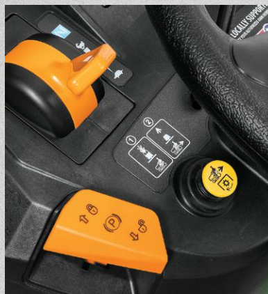
Electric PTO. Available on some models, provides instant engagement of mower blades. (available on all models from S130 and above).
