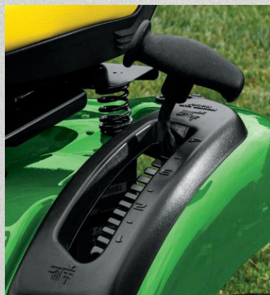
The convenient mower deck lift lever. ¼-in. (0.64-cm) height-of-cut increment adjustment is as precise as ever.
