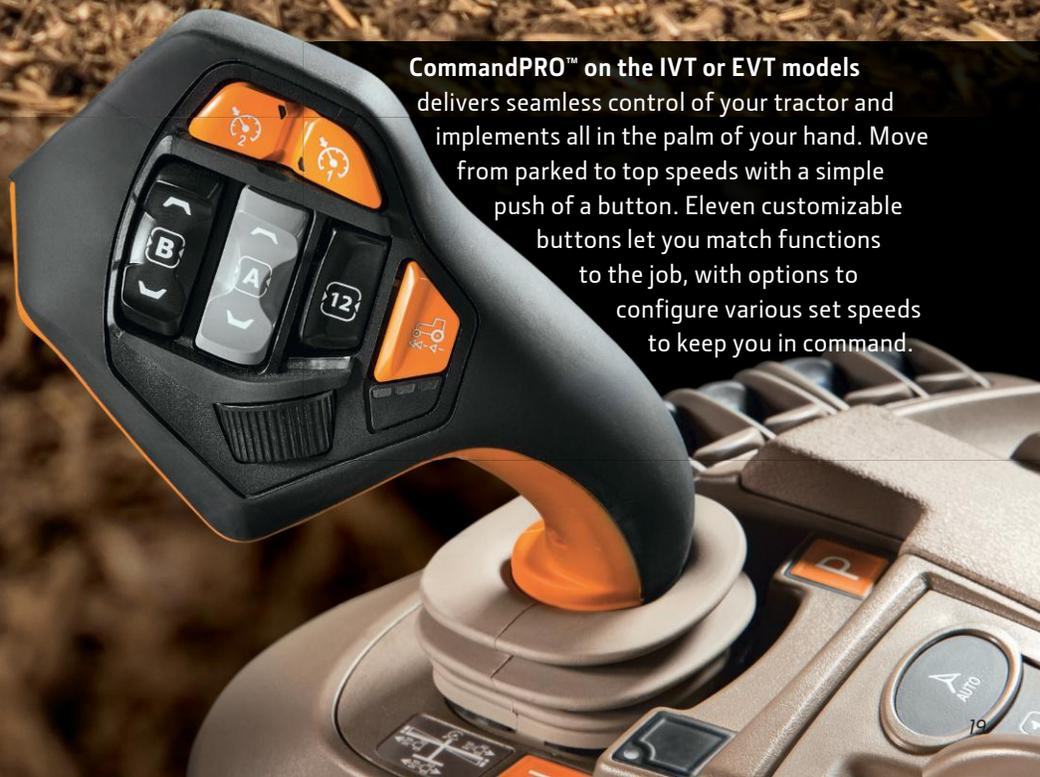
**CommandPRO™ on the IVT or EVT models** delivers seamless control of your tractor and implements all in the palm of your hand. Move from parked to top speeds with a simple push of a button. Eleven customizable buttons let you match functions to the job, with options to configure various set speeds to keep you in command.
