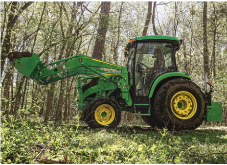
4075R Tractor with 440R Mechanical Self-Leveling Loader (MSL), cab, heat and A/C and pallet forks. See page 8.
