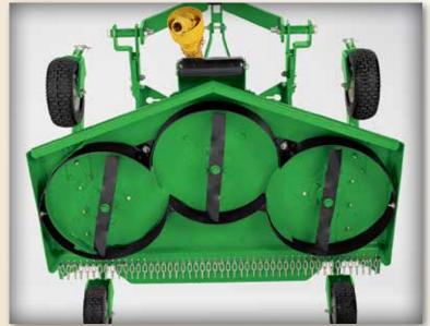
GM20 Series Mowers (pictured) have five blade options: standard, low-lift, high-lift, mulching and gator. The GM2190 and GM2109 have two free-swinging blades per rotor.
