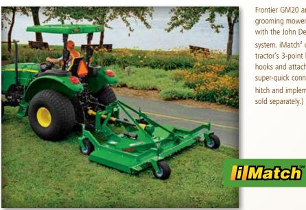
Frontier GM20 and GM21 Series grooming mowers can be fitted with the John Deere iMatch system. iMatch<sup>2</sup> converts your tractor's 3-point hitch to fixed hooks and attaching points for a super-quick connection. (iMatch hitch and implement A-frame kit<sup>3</sup> sold separately.)
