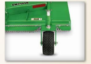
Stamped wheel yokes with pneumatic tires have spacers for quick and easy height adjustments.
