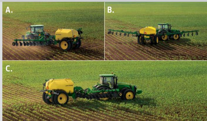
**Hydraulic wing kick** automatically lifts the wings higher than the main toolbar when turning in the field, providing increased clearance to greatly reduce any crop damage.
