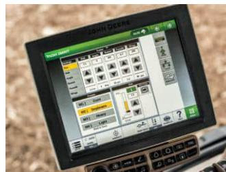
Change the depth of individual sections with **TruSet™ Side-Side** to accommodate varying field conditions and ensure proper product placement and sealing. Single-point depth control is included on all models as an easy adjustment to maintain depth across the entire machine.
