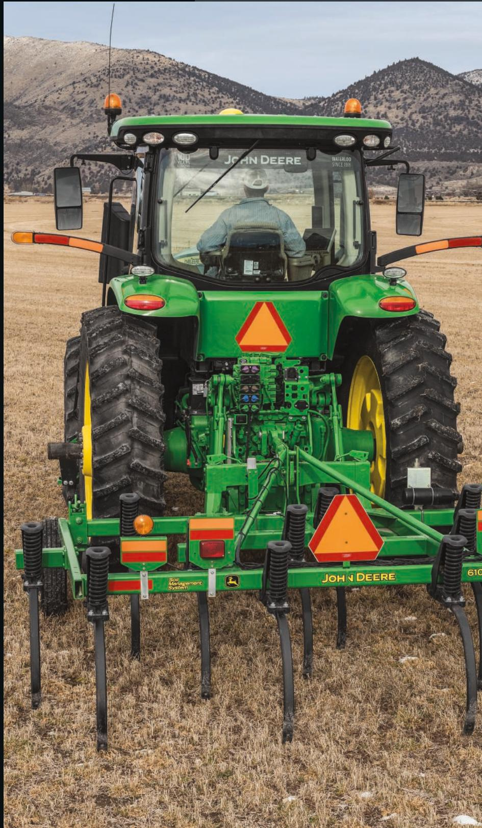
Get the soil breakup and shattering you demand from a chisel plow, plus excellent residue flow – with pick-up-and-go mobility with the 610 Integral Chisel Plow.
