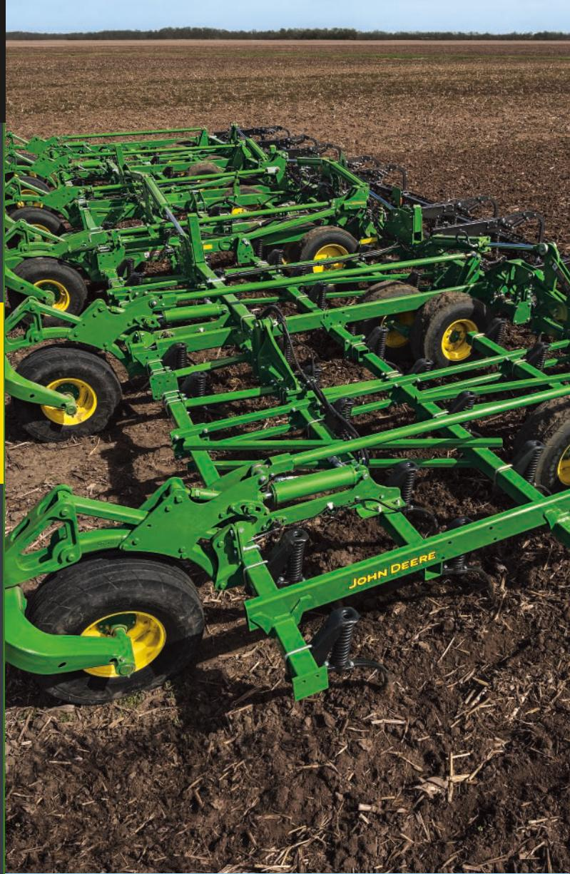
*The 2230FH Floating Hitch Field Cultivator works independently from the tractor and follows the contour of the ground so the implement remains level.*
