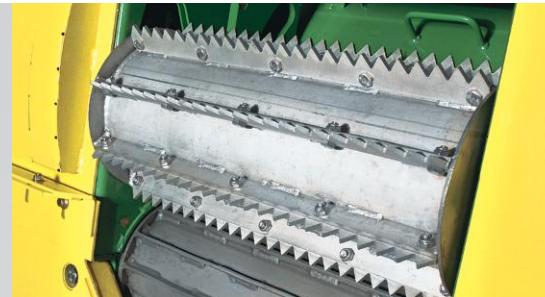
Save money with an upper front feedroll that features **bolt-on serrated or straight replaceable teeth bars** specifically designed for high wear conditions, sandy soil, and high-yield corn.
