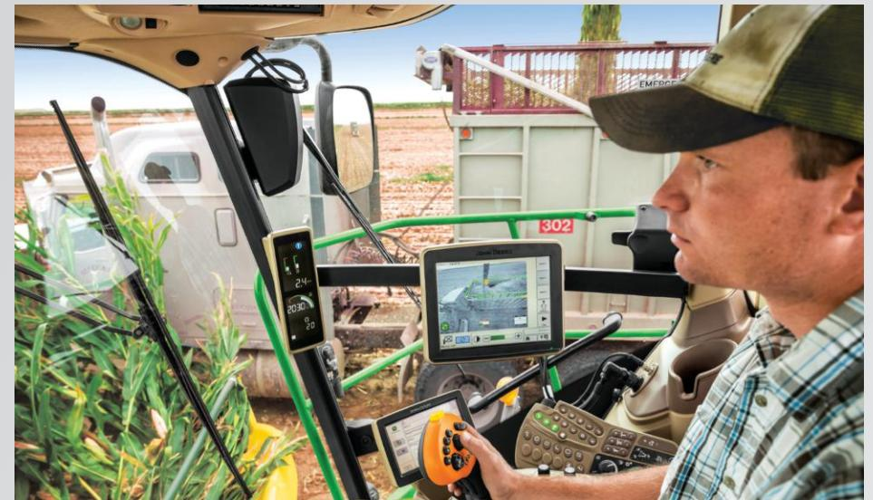
Ensure your crop doesn't end up on the ground. The optional Active Fill Control uses cameras with 3D capability to automatically detect the crop transport truck or trailer, and fill it evenly and without spillage. As the camera detects a truck, it automatically begins tracking with the spout. Then it controls the rotation and cap position of the spout until the truck is filled.
