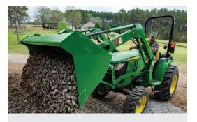
OPTIONAL 300E LOADER with a Mechancial Self Leveling Loader (MSL) option has a lift height of 84 in. (214 cm) and a lift capacity of 1283 lb (539 kg) measure at 19.7 in (500 mm) ahead of the pivot, so you can shoulder just about anything. Non Self-Leveling option available.
