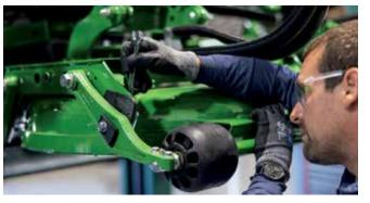
All height of cut adjustments on the 9009A can be performed with a single tool, and utilize an innovative notch system for precision and accuracy.
