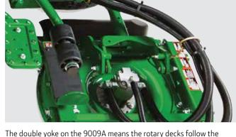
The double yoke on the 9009A means the rotary decks follow the contours in the most undulating terrain for an exceptional quality and consistency of cut.
