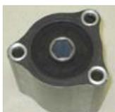
The torsion of each spring on the floor supports can be individually modified to adjust the flotation or to compensate for any unevenness in the cutterbar for true tailored harvesting performance.
