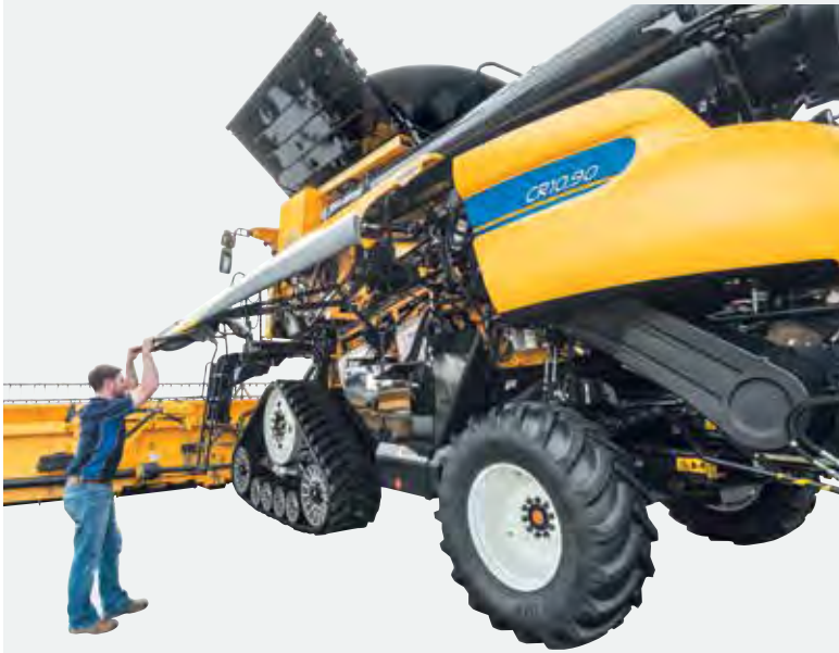
Easy ground-access to all oil filters and drain points and centralized greasing banks.
