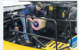
Access the air filter easily from the engine platform.
