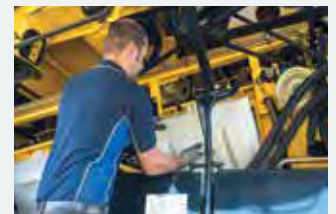
Plastic rotor covers can be removed without tools.
