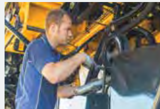
Easy ground-access to all oil filters and drain points and centralized greasing banks.
