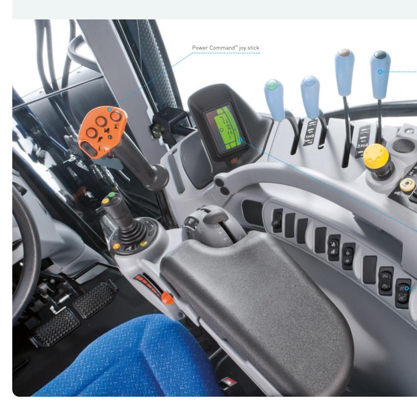
With the Classic armrest, you enjoy easy access to mechanical remote levers, PTO engagement, switches to control 4WD engagement, differential lock, auto shift range function, and more. You can also easily perform quick, clutch-free gear changes with the Power Command<sup>™</sup> joystick.
