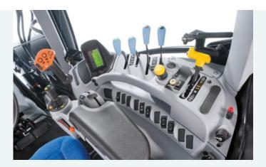
Value-focused Classic models with Range Command and Power Command transmissions are available with mechanical hydraulic remotes. The Classic armrest features easy-to-operate and logically and ergonomically positioned switches and controls.
