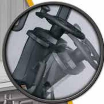
Yale Veracitor® VX forklift design goals include easy entry and exit, superior driver comfort, and ease of operation. The ergonomically designed 12" steer wheel with spin knob and infinitely adjustable steer column are shown.
