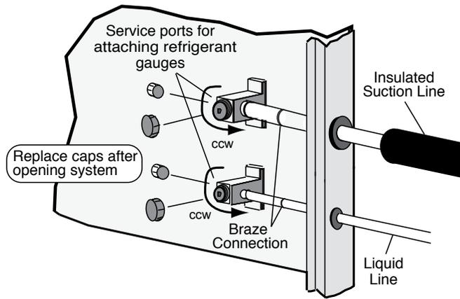
**Figure 14: Attaching the Air Coil**
