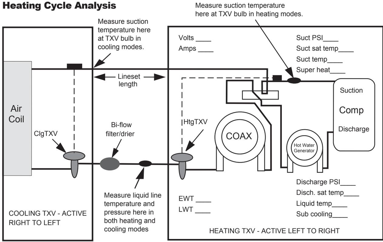
Heat of Extraction/Rejection = GPM x 500 (485 for water/antifreeze) x ΔT
