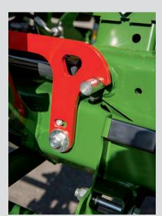
Automatically locked for transport Hydraulic check valves lock and release the mowers automatically when these are moved into work or transport position.
