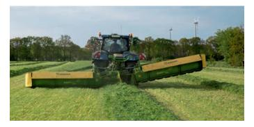
The mowers lift out separately as a standard feature Operators can raise one mower when cutting wedges. Simply select the mower that is not in work on the electric control box and raise it.
