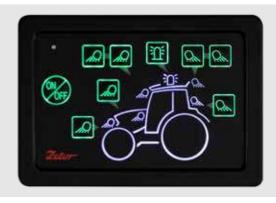
The tractor is equipped with a new controller for controlling work lights and beacons. It offers a number of advanced functions such as automatic activation of work lights according to the selected driving direction or a memory function.
