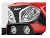
3. The use of new headlights allows illumination of a larger work area and offers higher luminosity.
